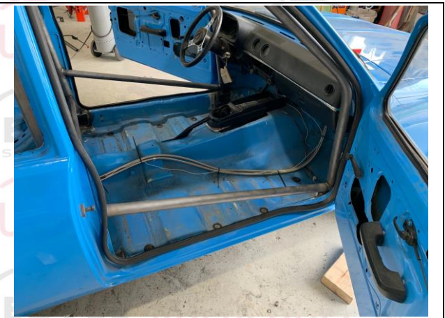
PHOTO 11 ANTI-INTRUSION DOORBAR – CO-DRIVER
