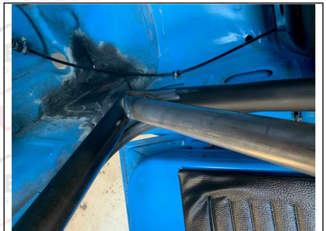
PHOTO 6 FRONT ROLLBAR TO FLOOR ATTACHMENT
