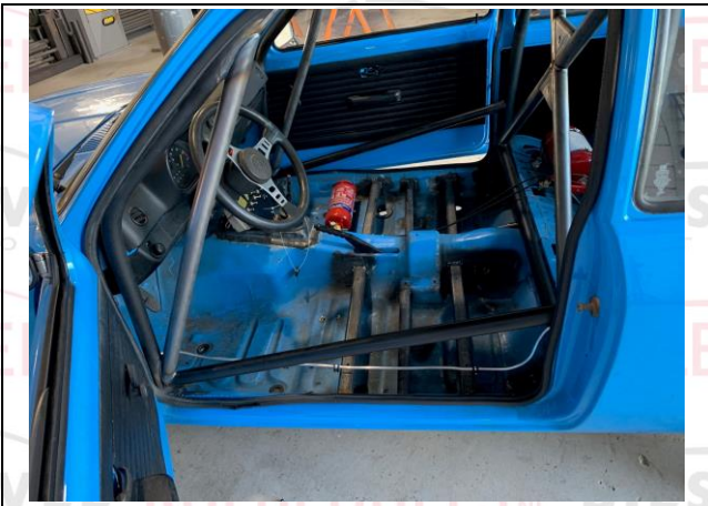
PHOTO 10 ANTI-INTRUSION DOORBAR - DRIVER
