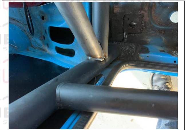
PHOTO 4 MAIN ROLLBAR TO FLOOR ATTACHMENT
